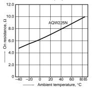
2.-(2) On resistance vs. ambient temperature characteristics
